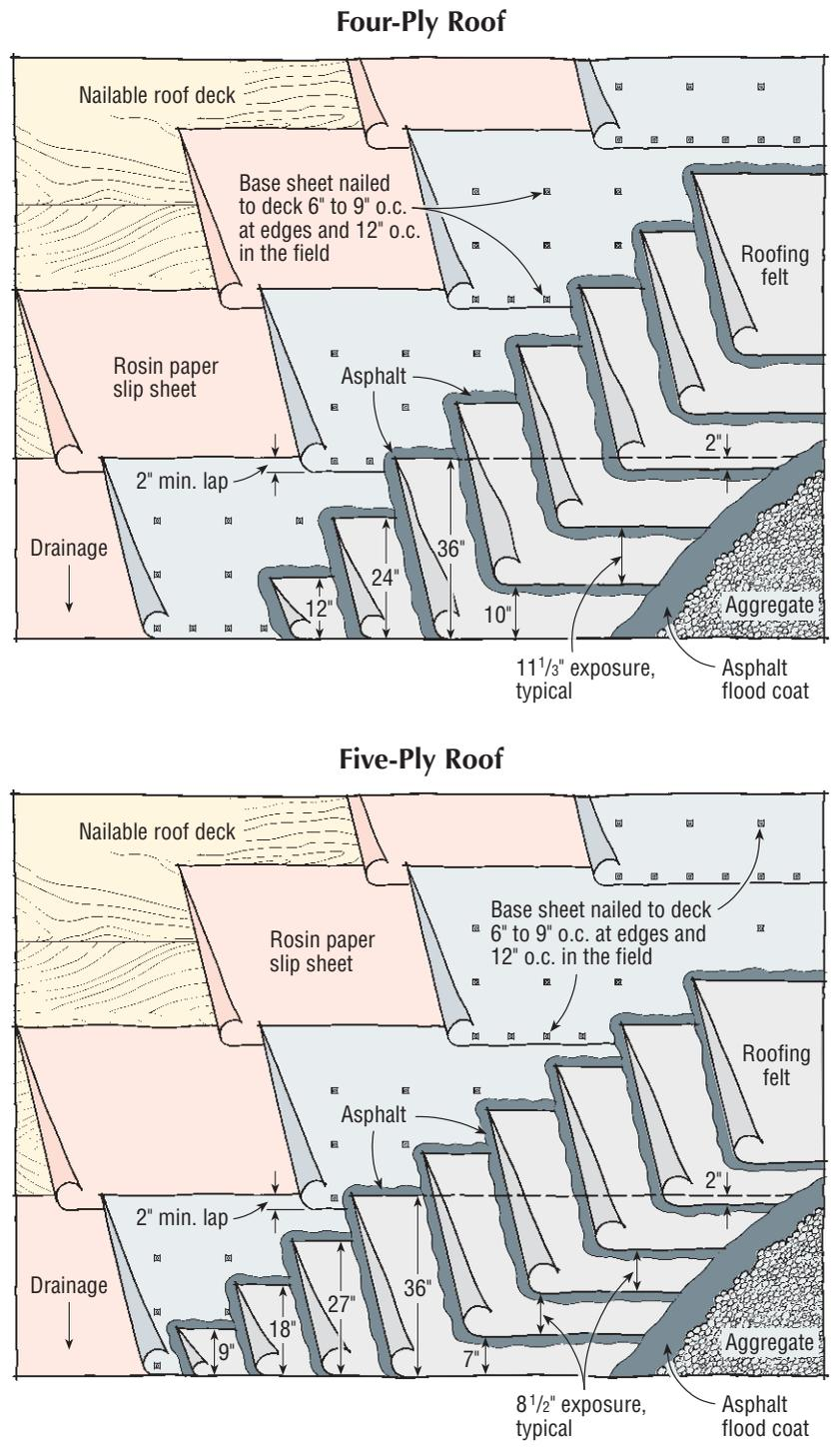
**Figure 9.** The same materials can be laid up different ways. Most residences have framed wood roofs, so the first waterproofing layer is a nailed-on base sheet. Successive layers of felt are bedded in hot asphalt and covered with a cap sheet, an emulsion coating, or, as is shown here, a flood coat of asphalt and loose aggregate. Because the base sheet qualifies as a layer, a base sheet plus three layers of mopped-in felt constitutes a four-ply roof.
