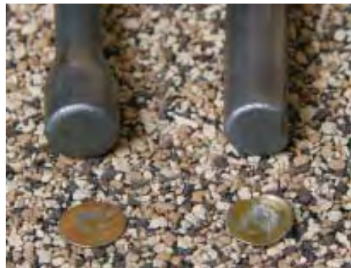
Figure 5. Until they get worn, round drivers like the one on the left make full contact with the nail, so the head is always driven flat. However, most roofing guns have asymmetrical drivers like the one on the right. Because these drivers do not make full contact with the nail, in some circumstances the head may deform so that one edge sticks up above the plane of the shingle.
