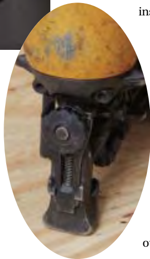
Figure 4. On most roofing nailers, depth-of-drive is adjusted by turning a thumb-wheel on the nose or near the trigger, as on the Senco gun (above). The depth-of-drive on the Bostitch (right) is especially easy to adjust because the mechanism is controlled by a large knob on the nose.
